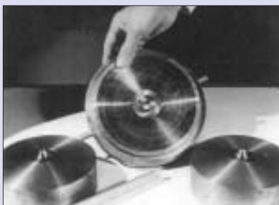
Below Tracey Hall's belt device played a key role in the synthesis of diamond Right Photo of the diamond crystals produced in the first successful run in December 1955
